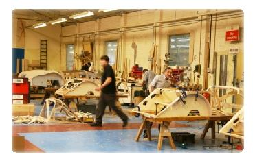
The surprise is that they are still built the same way. Once the steel frame is laid out, most of the rest of the car is made of wood secured by jigs and templates still in use over decades.
