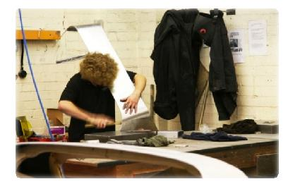
The metal parts, like body panels, doors and fenders, are formed bent and hammered into shape by men who know the exact curve a hood has to be to go on the car. No wonder replacement parts are so expensive.
