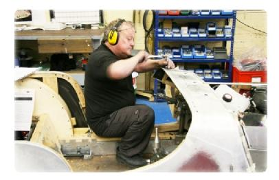
Other body parts are screwed and nailed to the wooden frame and by the time it rolls into the trim shop you cannot see any trace of the original ash framing.
